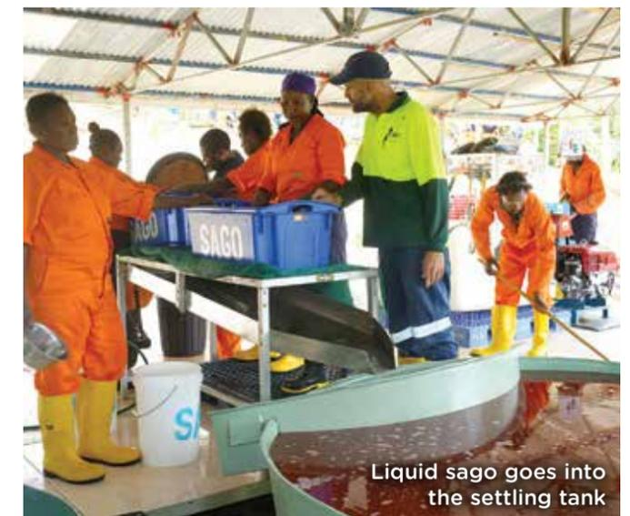
Liquid sago goes into the settling tank
